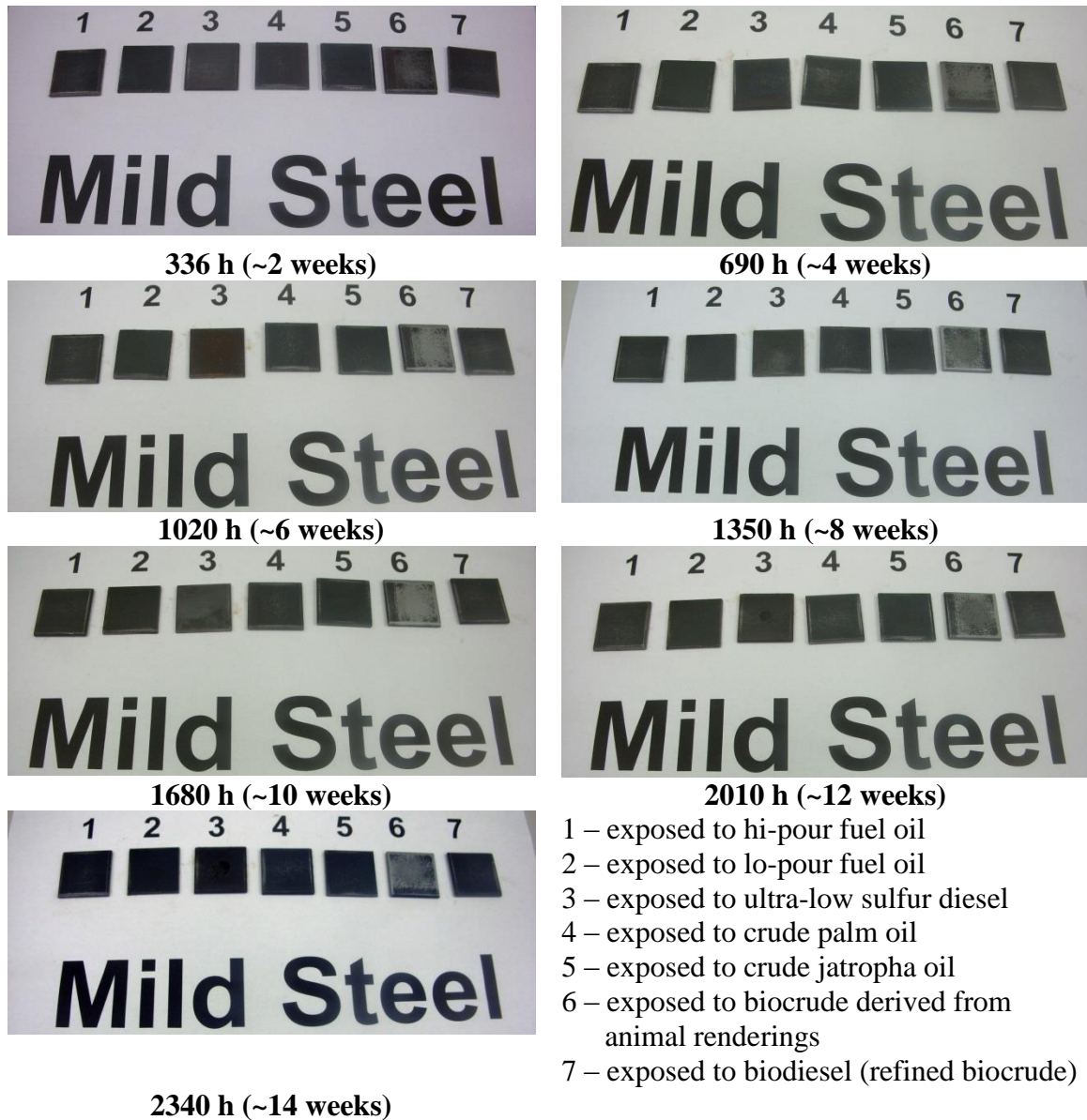
Figure 7-133. Mild steel samples after exposure to pure oils.
