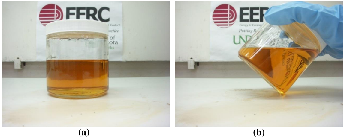
Figure 7-92. Crude jatropha oil – biodiesel blend, cooled from 220°F to 75°F. (a) shows the blend sitting flat, and (b) shows the blend tilted at an angle.
