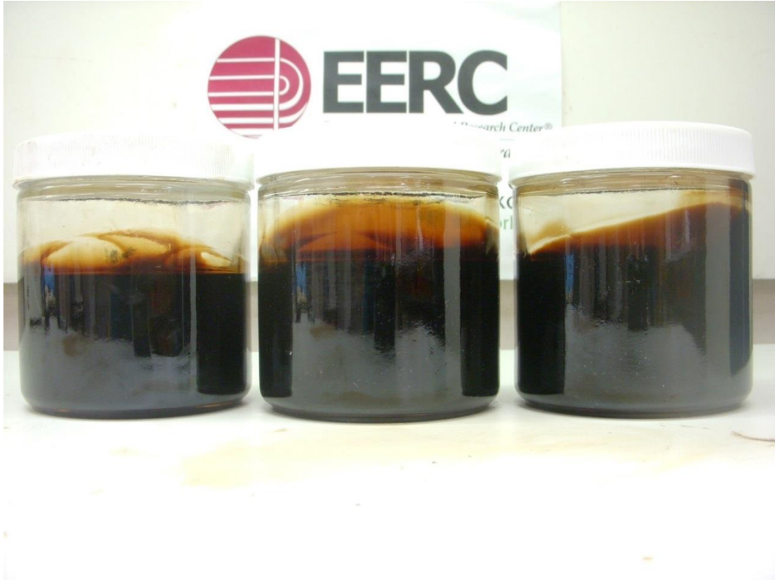
Figure 7-99. Hi-pour fuel oil – biodiesel blend. In order from left to right, original blend temperatures were 75°F, 170°F, 220°F. All blends have been photographed at 75°F.
