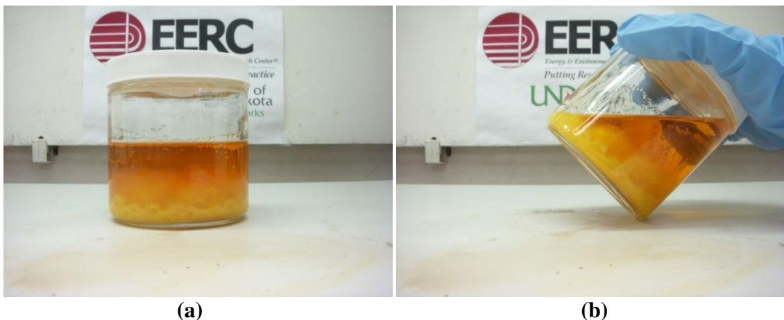
Figure 7-90. Crude palm oil – ultra-low sulfur diesel blend, cooled from 220°F to 75°F. (a) shows the blend sitting flat, and (b) shows the blend tilted at an angle.
