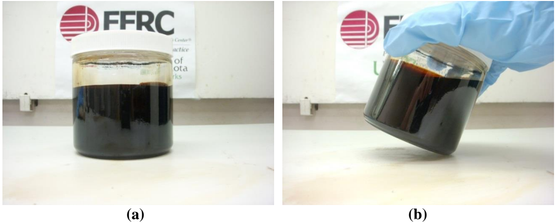
Figure 7-59. Hi-pour fuel oil – crude jatropha oil blend, cooled from 170°F to 75°F. (a) shows the blend sitting flat, and (b) shows the blend tilted at an angle.
