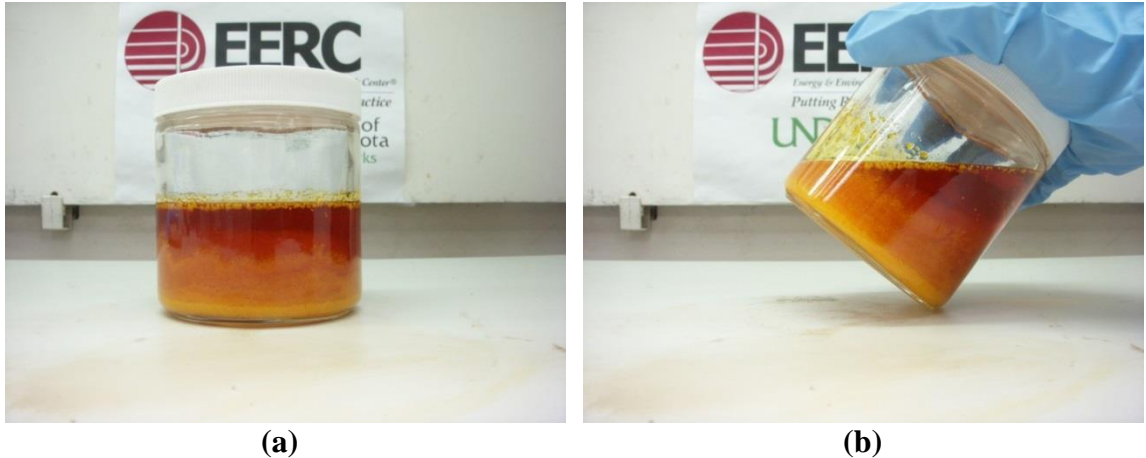
Figure 7-70. Crude palm oil – biodiesel blend, cooled from 170°F to 75°F. (a) shows the blend sitting flat, and (b) shows the blend tilted at an angle.
