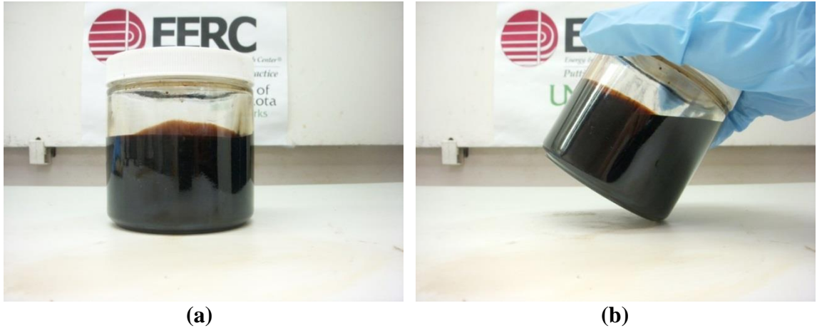
Figure 7-62. Hi-pour fuel oil – ultra-low sulfur diesel blend, cooled from 170°F to 75°F. (a) shows the blend sitting flat, and (b) shows the blend tilted at an angle.
