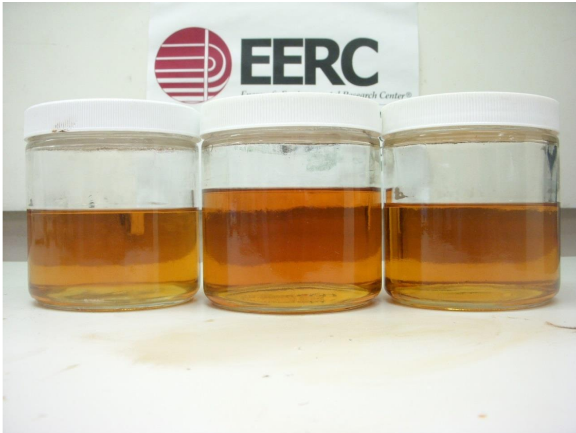
Figure 7-111. Crude jatropha oil – biodiesel blend. In order from left to right, original blend temperatures were 75°F, 170°F, 220°F. All blends were photographed at 75°F.
