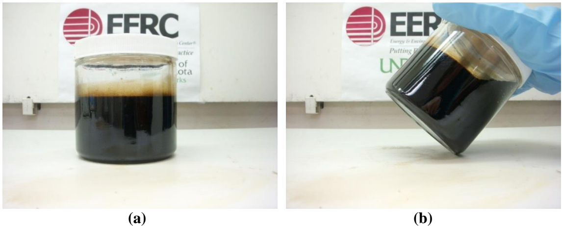
Figure 7-82. Lo-pour fuel oil – crude palm oil blend, cooled from 220°F to 75°F. (a) shows the blend sitting flat, and (b) shows the blend tilted at an angle.
