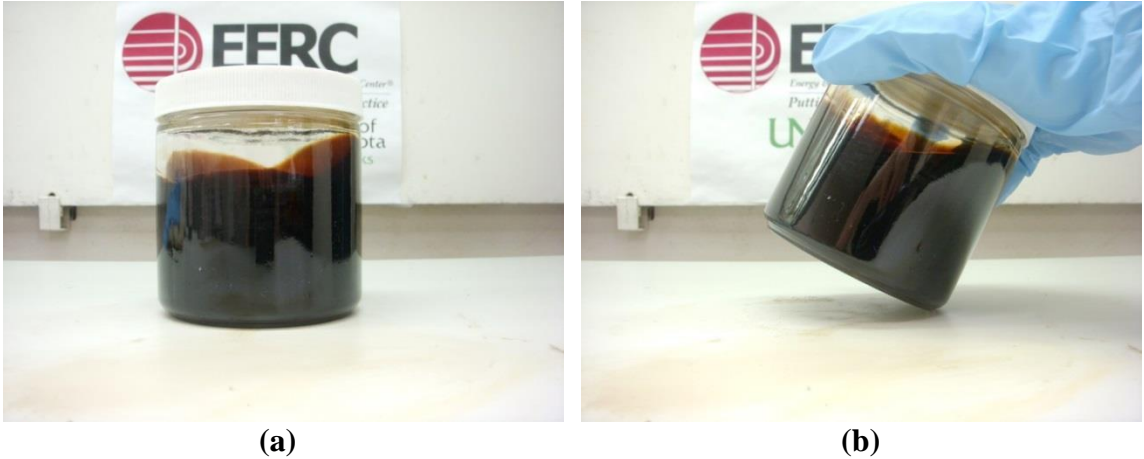
Figure 7-61. Hi-pour fuel oil – biodiesel blend, cooled from 170°F to 75°F. (a) shows the blend sitting flat, and (b) shows the blend tilted at an angle.
