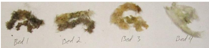
Figure 3-5. Tars collected on filter media.
