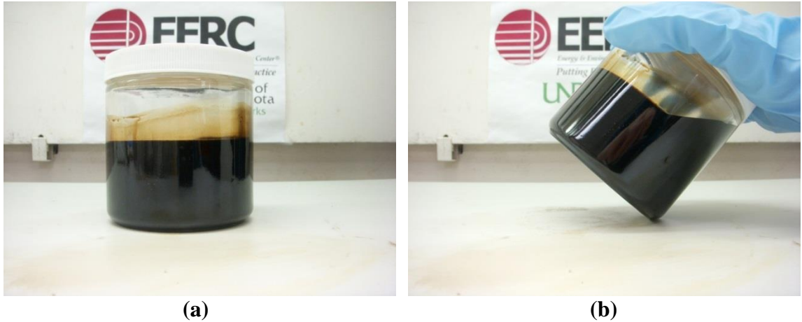
Figure 7-84. Lo-pour fuel oil – biocrude blend, cooled from 220°F to 75°F. (a) shows the blend sitting flat, and (b) shows the blend tilted at an angle.
