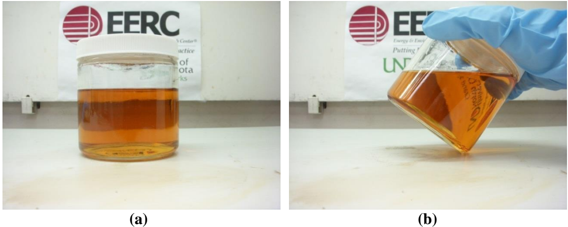
Figure 7-73. Crude jatropha oil – biodiesel blend, cooled from 170°F to 75°F. (a) shows the blend sitting flat, and (b) shows the blend tilted at an angle.
