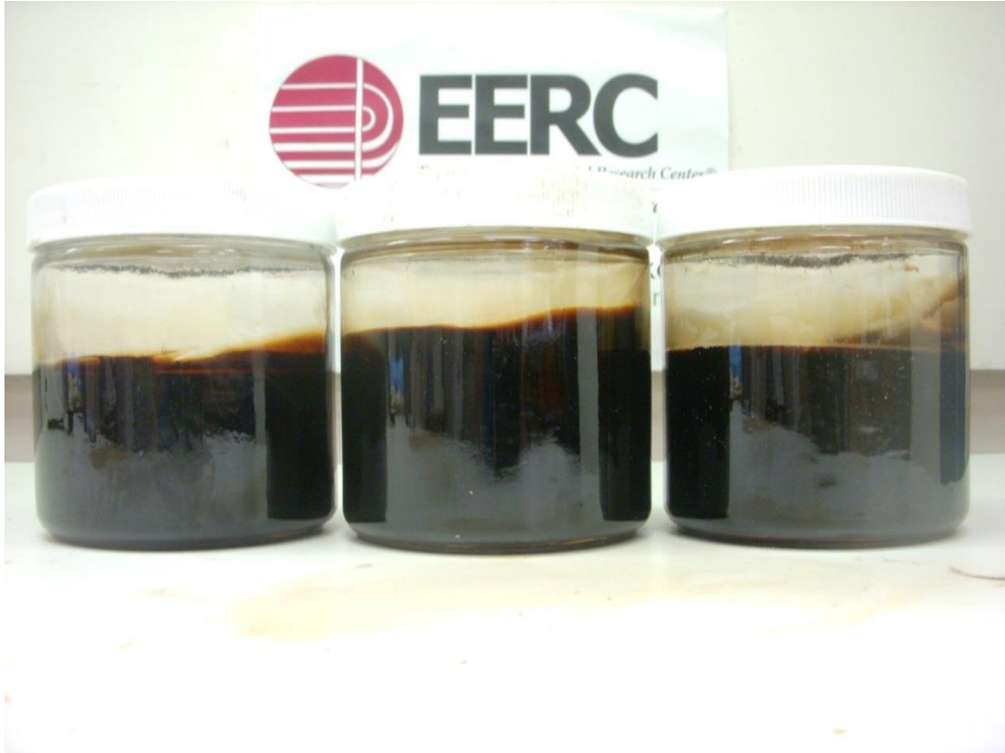
Figure 7-104. Lo-pour fuel oil – biodiesel blend. In order from left to right, original blend temperatures were 75°F, 170°F, 220°F. All blends were photographed at 75°F.
