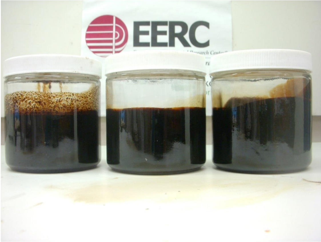
Figure 7-98. Hi-pour fuel oil – biocrude blend. In order from left to right, original blend temperatures were 75°F, 170°F, 220°F. All blends have been photographed at 75°F.
