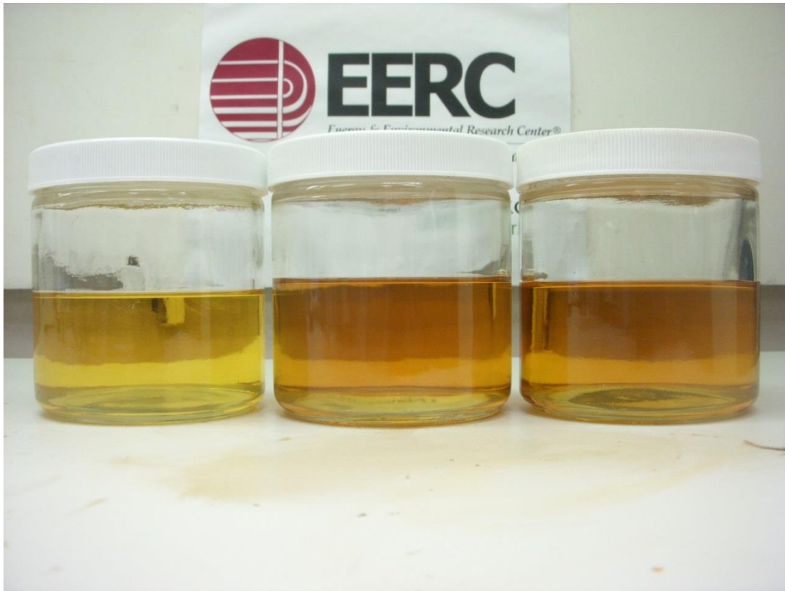
Figure 7-114. Biodiesel – ultra-low sulfur diesel blend. In order from left to right, original blend temperatures were 75°F, 170°F, 220°F. All blends were photographed at 75°F.
