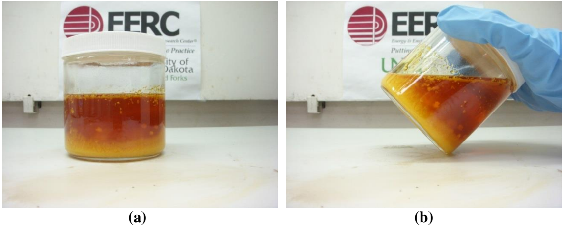
Figure 7-89. Crude palm oil – biodiesel blend, cooled from 220°F to 75°F. (a) shows the blend sitting flat, and (b) shows the blend tilted at an angle.
