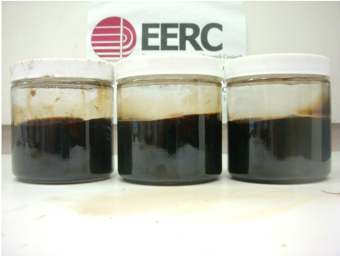
Figure 7-105. Lo-pour fuel oil – ultra-low sulfur diesel blend. In order from left to right, original blend temperatures were 75°F, 170°F, 220°F. All blends were photographed at 75°F.
