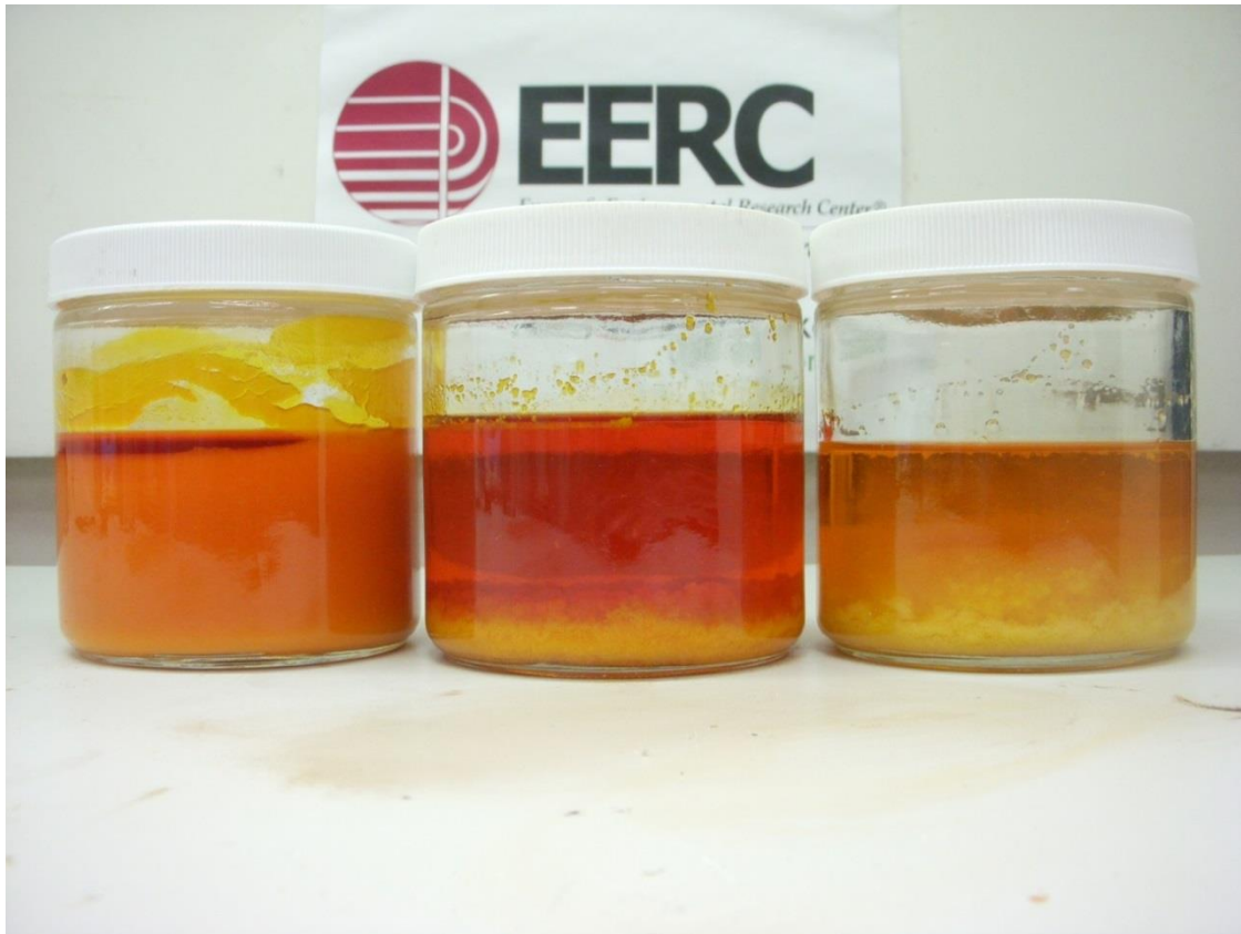
Figure 7-109. Crude palm oil – ultra-low sulfur diesel blend. In order from left to right, original blend temperatures were 75°F, 170°F, 220°F. All blends were photographed at 75°F.
