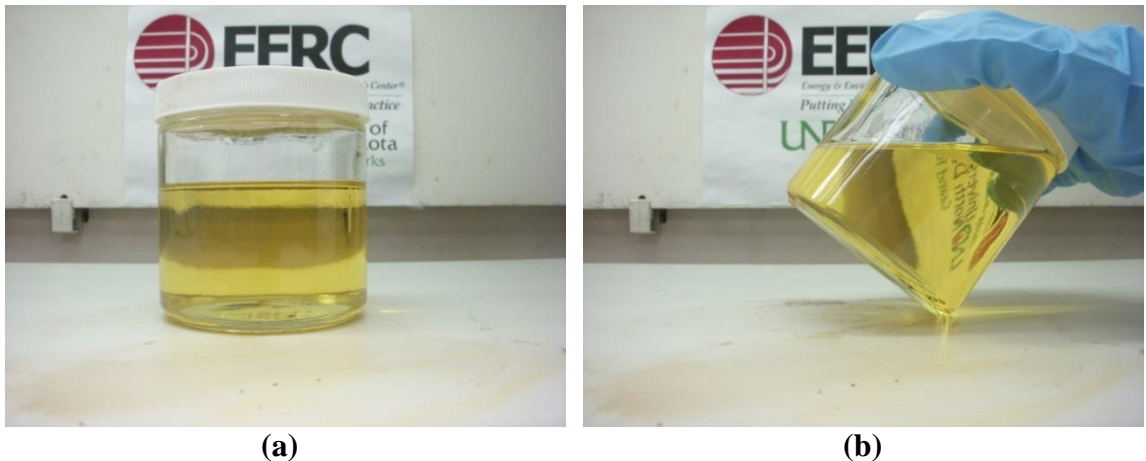
Figure 7-93. Crude jatropha oil – ultra-low sulfur diesel blend, cooled from 220°F to 75°F. (a) shows the blend sitting flat, and (b) shows the blend tilted at an angle.
