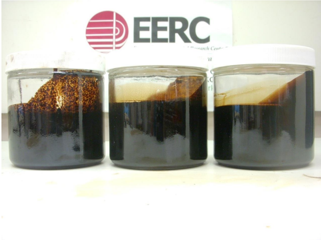
Figure 7-103. Lo-pour fuel oil – biocrude blend. In order from left to right, original blend temperatures were 75°F, 170°F, 220°F. All blends were photographed at 75°F.
