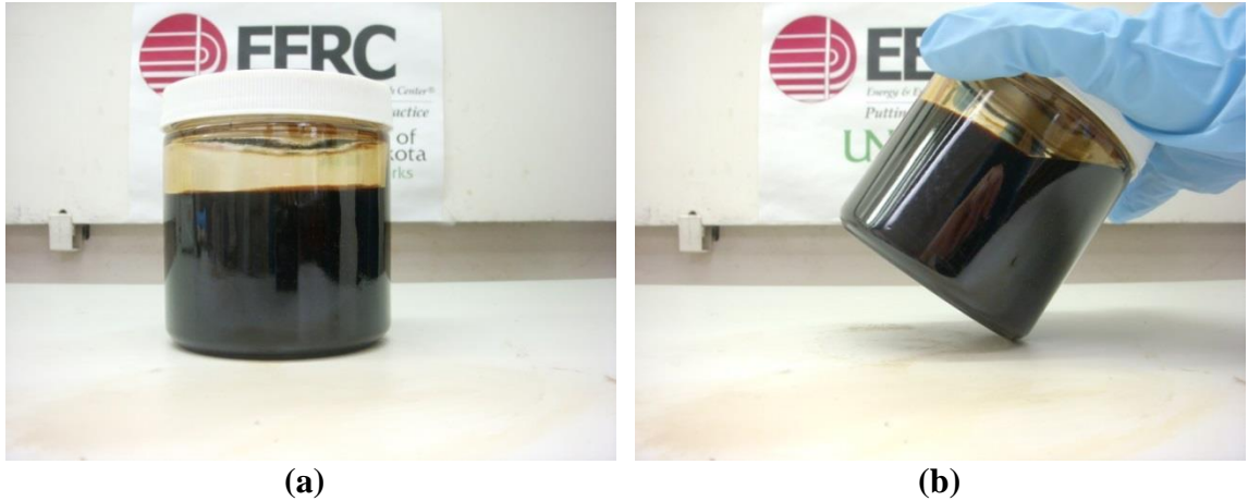
Figure 7-78. Hi-pour fuel oil – crude jatropha oil blend, cooled from 220°F to 75°F. (a) shows the blend sitting flat, and (b) shows the blend tilted at an angle.
